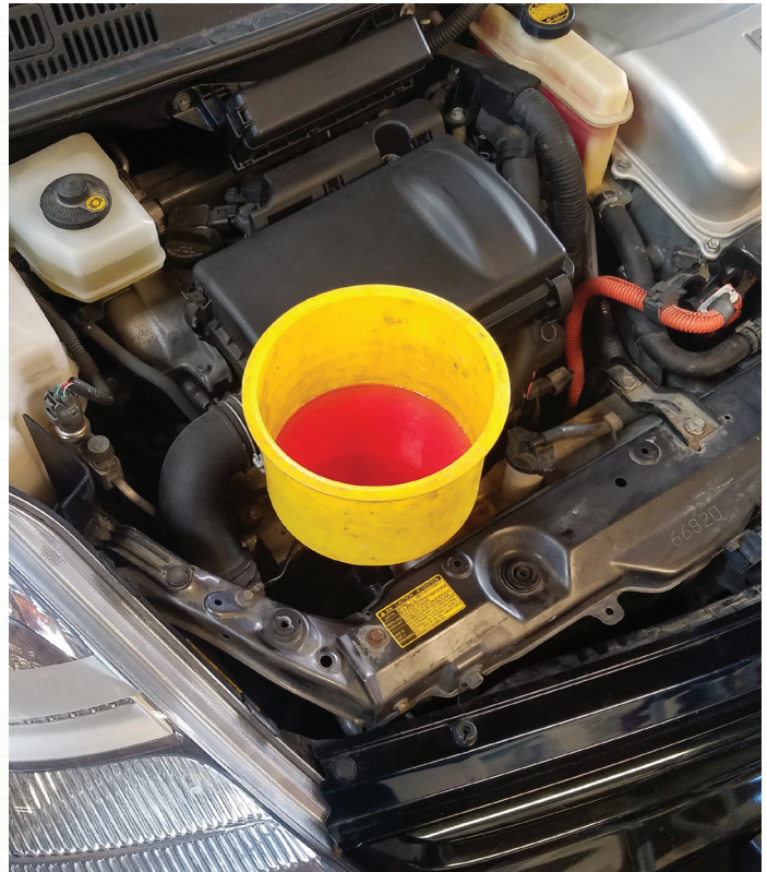
Fill and bleed the system with a bucket atop the radiator neck.
