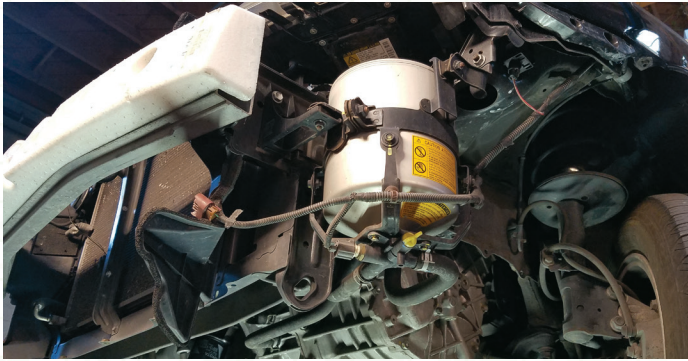
The Prius has a coolant thermos, or “Coolant Heat Storage” (CHS) tank located behind the front bumper.
