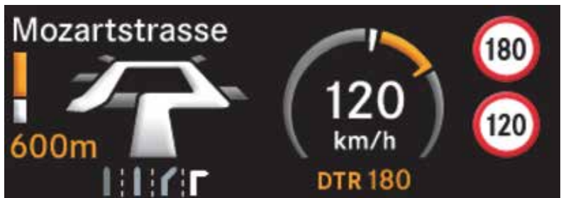
The head-up display test image 1 is an example of the typical layout of information as it would be projected onto the windshield for the driver.
