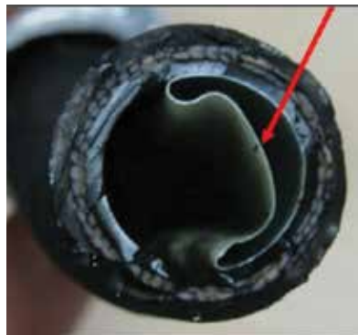
The inside of this suction hose has collapsed, causing a blockage, resulting in high low-side pressure readings and poor performance. Photo courtesy of Daimler AG.
