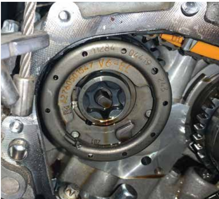
To remove the massive tamper-proof Torx bolt/control valve on the camshaft adjusters, you'll need Mercedes-Benz special tool W271 589 00 10 00.
