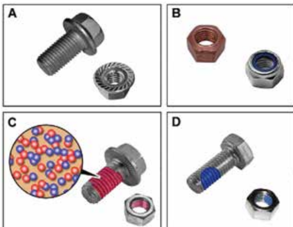
The four major types of self-locking fasteners: A) Locking splines B) Self-locking nuts C) Microencapsulated and D) Polyamide coating. See the text for details on handling each type.
