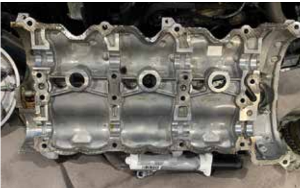
The valve cover castings also serve as the upper camshaft bearings. To prevent damage to the camshaft, mounting a special hold-down tool set (W276 589 01 40 00) is required before removing the chain tensioner.
