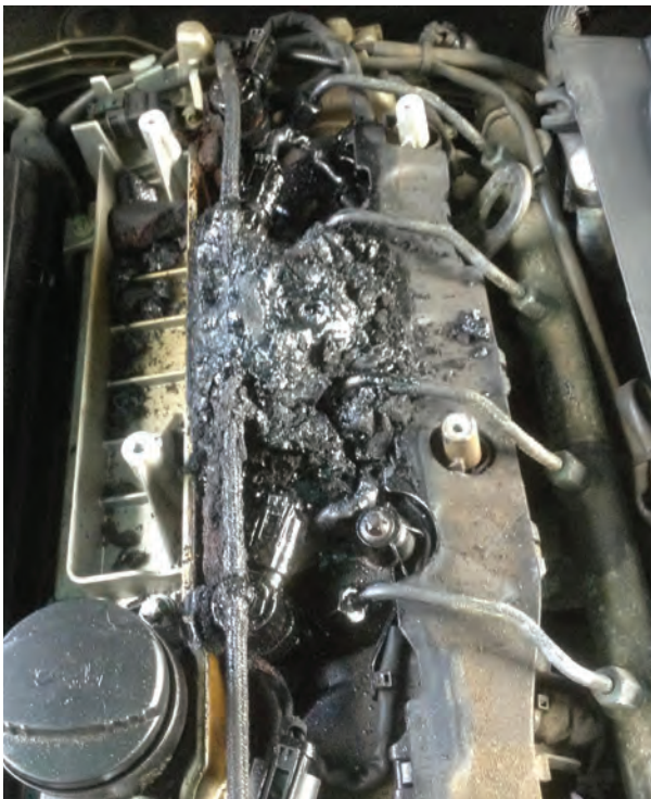
A severe case of Black Death. Removing the hardened carbon buildup is the first task.
