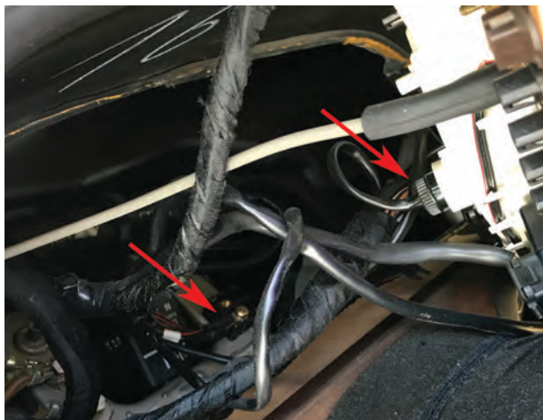
The upper arrow points to the vehicle speed signal output connector from the speedometer, the lower arrow points to the connector block for that signal.
