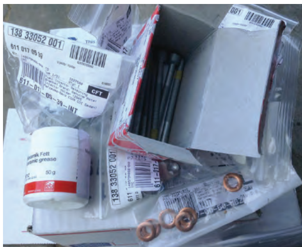
Some of the supplies you'll need to re-seal the fuel injectors: Seals, hold-down bolts and injector grease.
