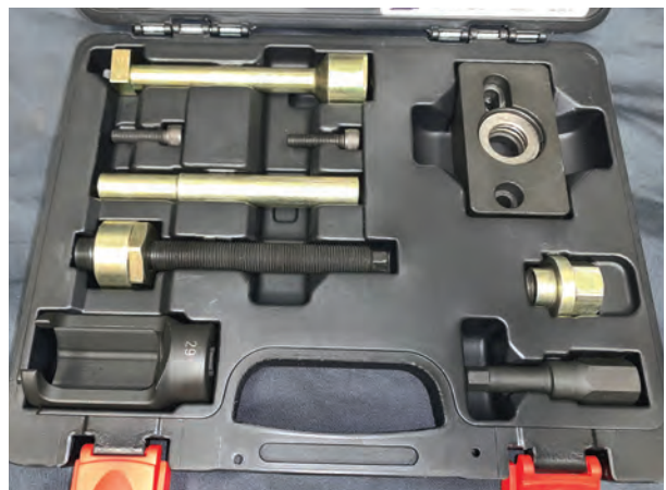
A typical injector puller set. Similar tools are available from several suppliers.
