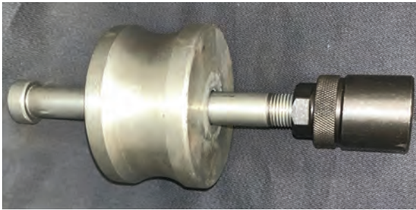
A slide hammer puller, here shown with a screw-on adaptor, works well if you have enough clearance.
