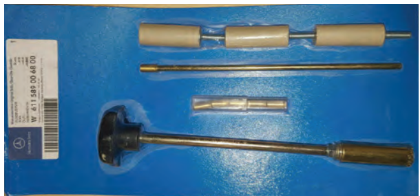
Clean the fuel injector bores using the proper tools.
