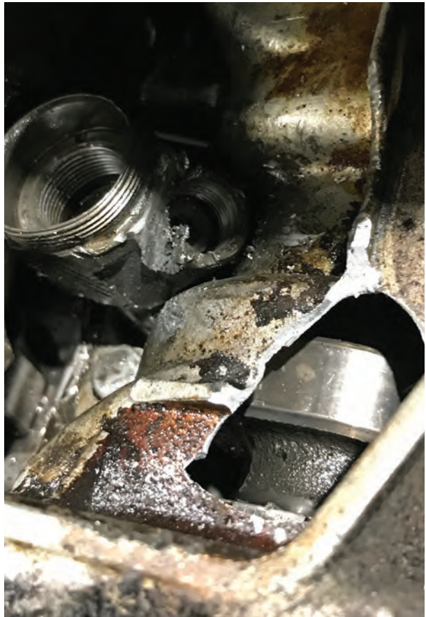
Beware of cracking the cylinder head cover if you use it as leverage to pry against!
