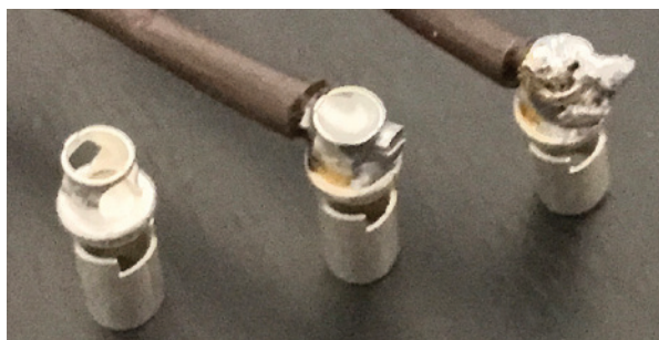
Three contacts (A003 545 26 26): one brand new, one properly soldered, and one cold-soldered. The cold-soldered contact is likely to fail if not re-soldered correctly.
