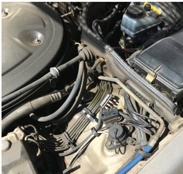
The 8-pole electrical connector (here seen unplugged) for the cruise control actuator is found next to the round diagnosis connector in this 1988 300SE.
