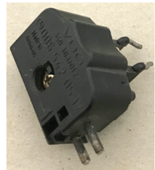
The electronic sensor used to generate the cruise control's vehicle speed signal in vehicles equipped with a mechanical speedometer. The inductive version shown has been replaced by an electronic version using a hall-effect sensor.
