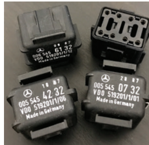
A few different reference resistors (coding plugs) that are used with the digital cruise control amplifier to match the system characteristics to the vehicle.
