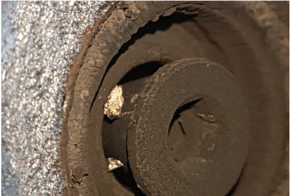
EGR stuck open
