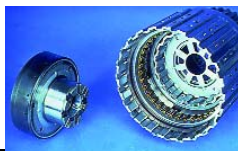
Overrunning Clutch Hub Installed
