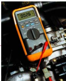
Figure 4 Measuring Primary Resistance Between Terminals 2 and 3
