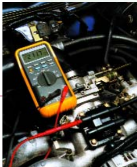
Figure 2 Measuring Secondary Resistance Between Terminals 3 and 4
