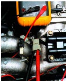
Figure 3 Measuring Primary Resistance Between Terminals 1 and 2
