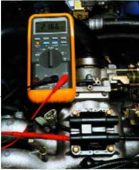
Figure 1 Measuring Secondary Resistance Between Terminals 1 and 2
