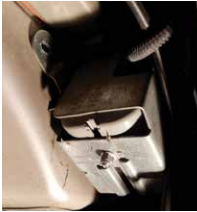
The alarm module or siren is located under the inner fender at the passenger side front
