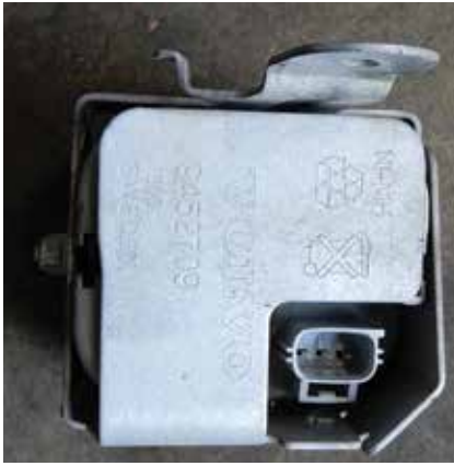
The alarm module or siren is located under the inner fender at the passenger side front
