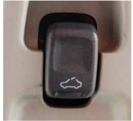
Sunroof button pushed to tilt the back of the sunroof open
