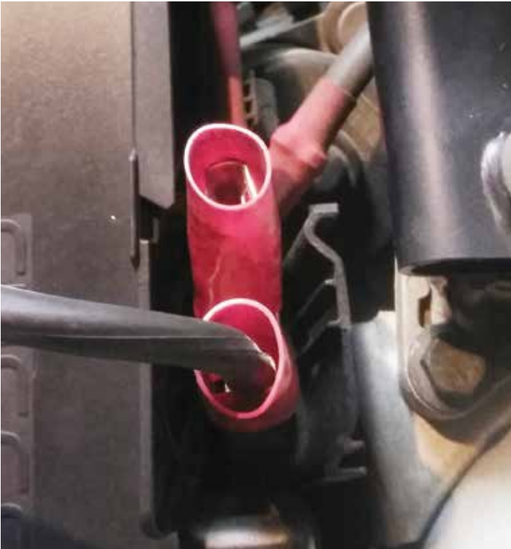
When checking or charging the battery on a Volvo, it's best to hook up at the battery; don't just hook up at the remote B+ at the fuse box; these connections are designed to be used for jump starting only.
