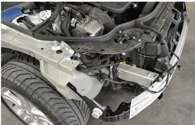
The Mercedes-Benz front crash module bolts onto the upper and lower frame rails (longitudinal members) on this 2010 GL 450. Mercedes-Benz Base certification training teaches the proper procedures for sectioning or replacing the structural components.
