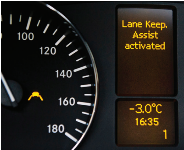
Instrument cluster messages let the driver know when the Lane Keeping Assist system is active, as shown here on the 2013 and up Sprinter.
