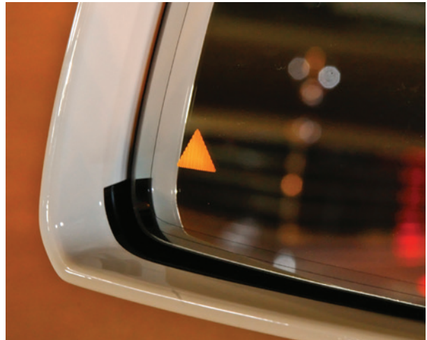
An orange triangular icon pops up on the appropriate side mirror to help alert the driver where not to go.
