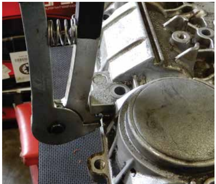
Using special tool 9995670 pliers to remove valve cover
