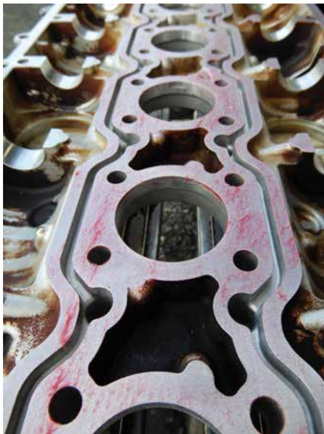
Apply liquid gasket to the valve cover with a roller.
