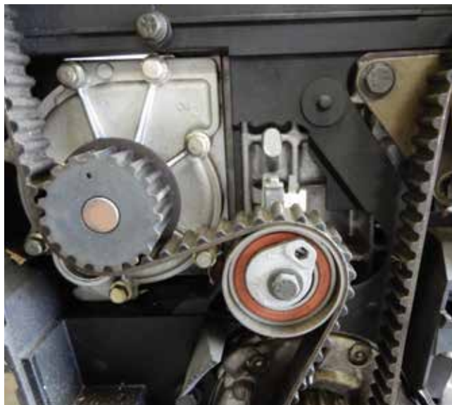
Timing belt tensioner in correct position
