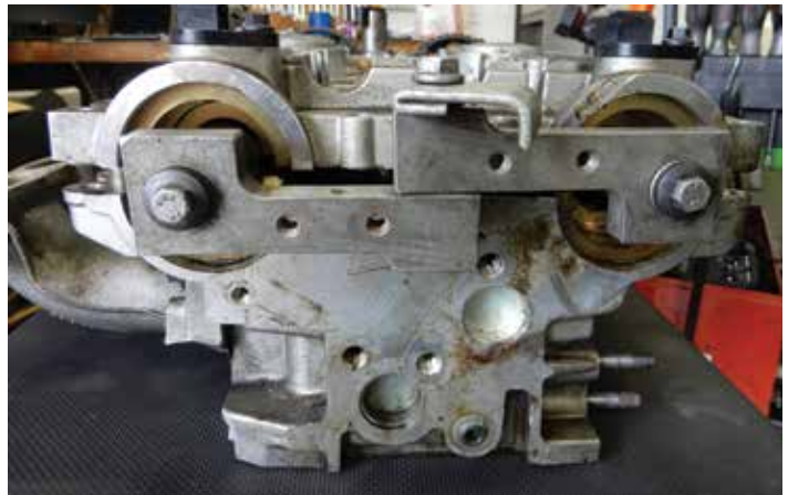
Tool installed at rear of camshafts
