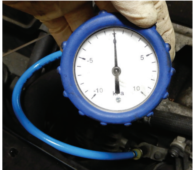
Volvo tool to check pressure in crankcase
