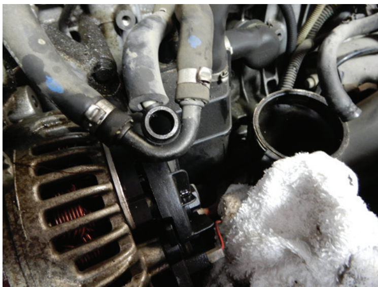
Banjo fitting at bottom of intake manifold
