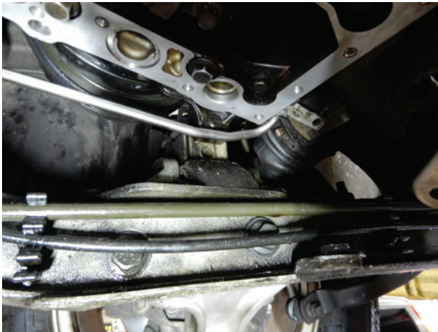
Engine mount with bolt in bottom mount threaded hole to lift engine up
