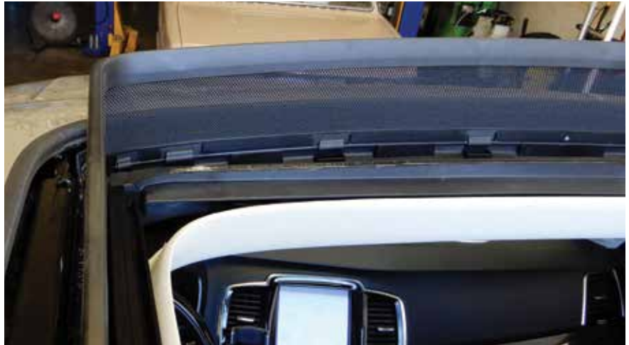
Laminated panoramic sunroof and front wind deflector
