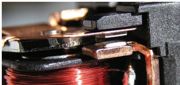
The square electrical contacts of this relay do most of the hard work, but they are not the only thing that can go bad.
