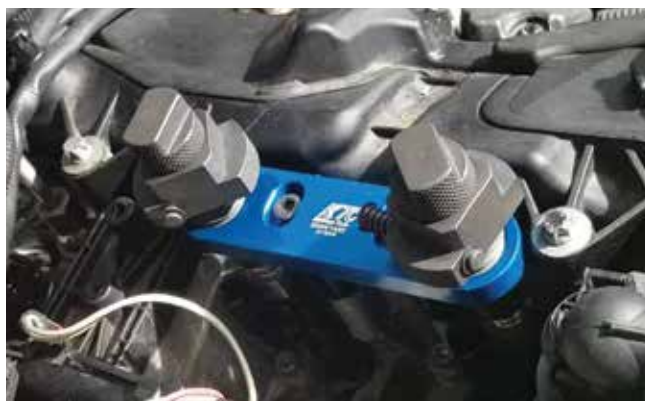
This removal and installation tool is needed for the N55 engine. With N54 engines you can use the slide hammer type puller.
