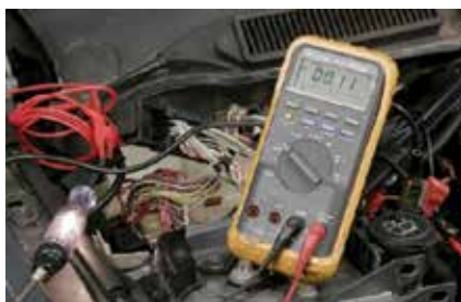
You should have 0.2 V or less when checking the voltage drop of the injector circuit. (Courtesy Opus IVS™)
