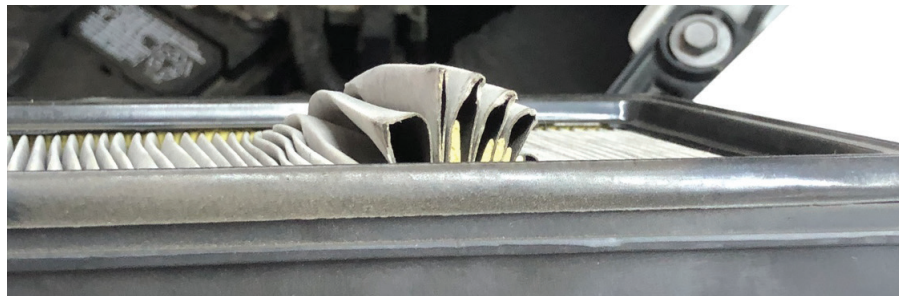
Figure 7: Broken air filter
