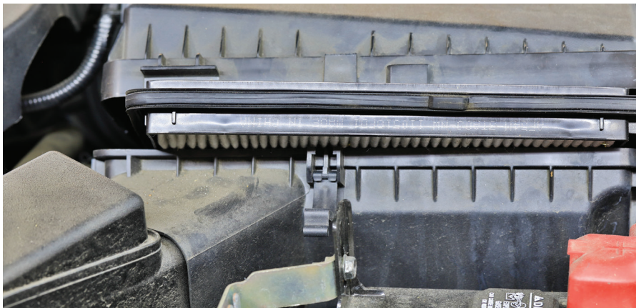
Figure 3: 2017 Altima air filter housing
