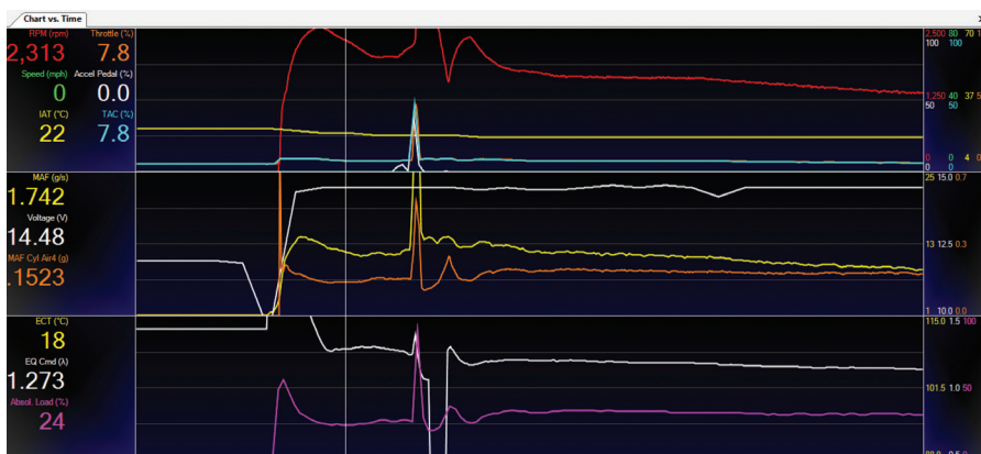
Figure 10: Cold start up with new MAF sensor
