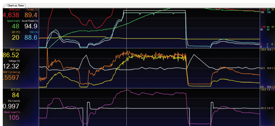
Figure 12: MR20DD VE test data
