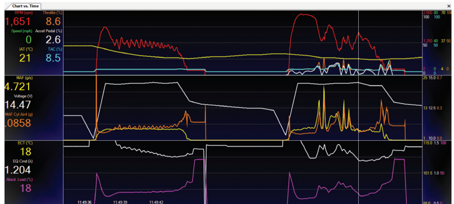
Figure 6: Start/Stall MAF sensor with throttle
