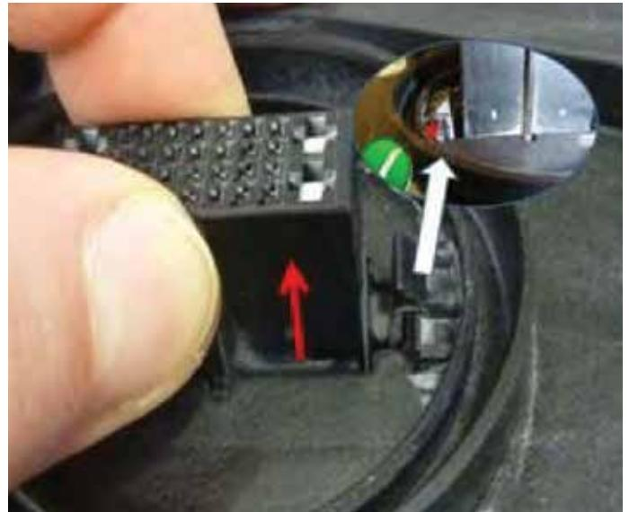
*Lift the connector up until you hear a clicking sound. The click means the locking tab has engaged and the connector is properly and securely positioned.*
