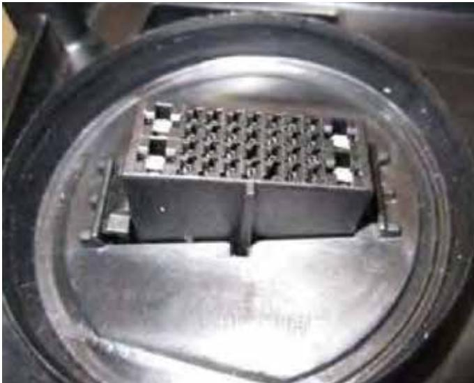
*On the LED headlight, check to confirm that the connector is down to the position shown in the picture. If it is not, push the connector all the way down.*
