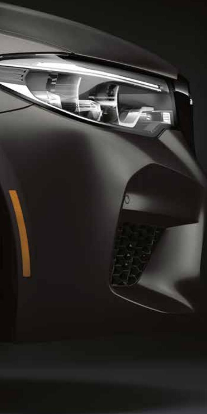
BMW Intelligent Headlight systems feature adaptive lighting technology that responds to different driving conditions. The state-of-the-art lighting provides better illumination for night driving, highlights pedestrians and potential obstacles in the road and, depending on the BMW model, reduces glare into the eyes of oncoming drivers.
