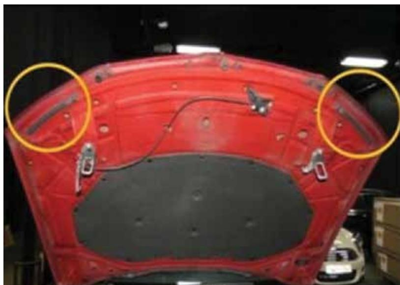
*Replace the old design seals (see yellow circles) on the left and right sides of the hood front lip with new dual-chamber reinforced sealing.*
