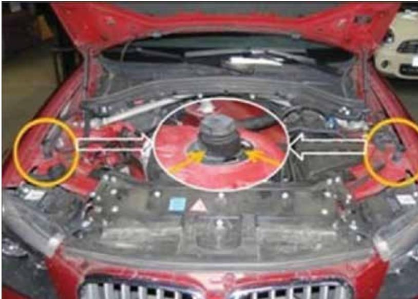
*If bump stops (pedestrian protection buffers, circled in yellow) are damaged or incorrectly positioned, they may allow the front end of the hood to press down excessively on the headlight housings, causing cracks and fissures in the lens covers.*
