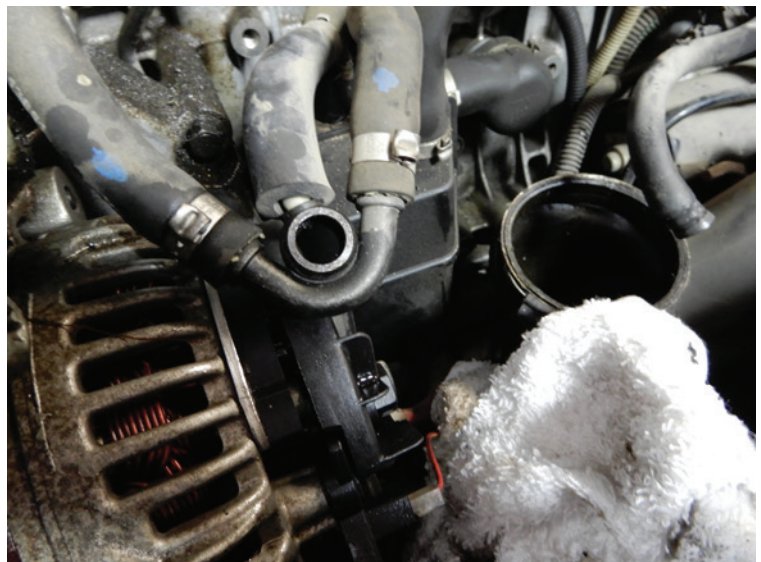
Banjo fitting at bottom of intake manifold
