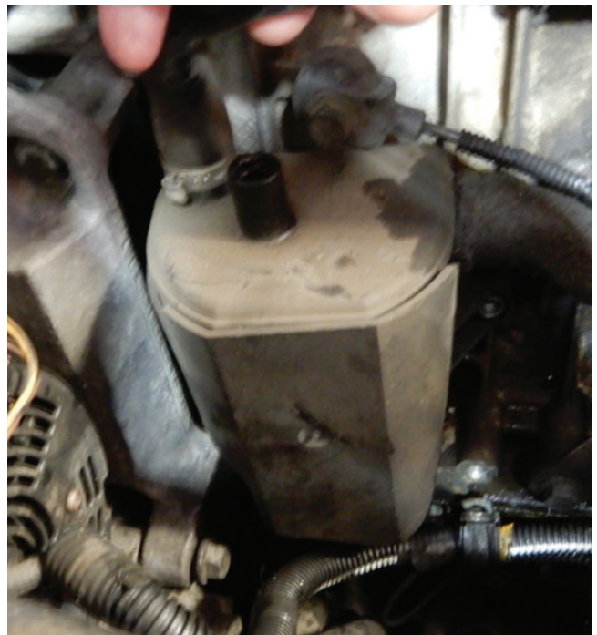
Volvo engine with intake removed and oil trap easy to see
