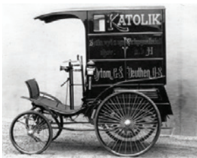
One of the earliest Benz delivery vans from 1896. The resemblance of the controls to those of the 1886 Patent Motorwagen is clear.
