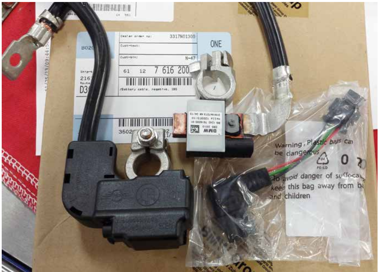
New generation IBS next to the old generation IBS.
