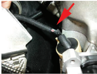
This harness is under tension and has damaged the electrical connector. After replacing the connector, re-route the wires to be completely tension-free.
