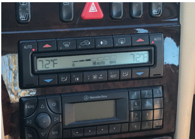
The climate control controller (N22) is located just above the radio in the center stack. Use the standard radio-removal tools to remove N22 from the dash.
