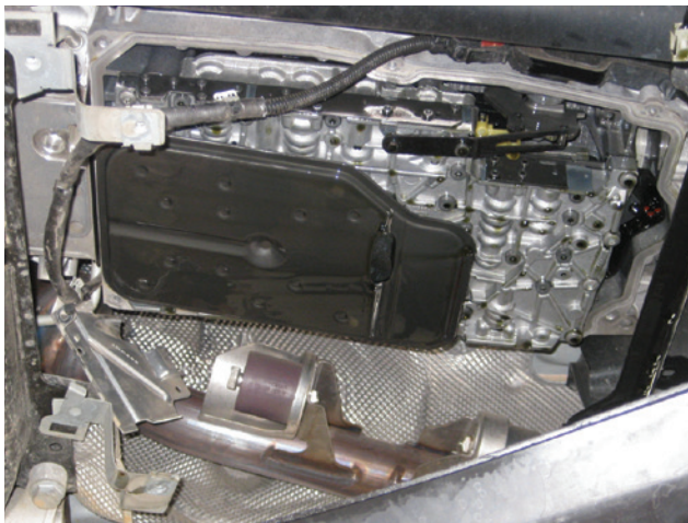
The VGS control unit is accessed by removing the transmission oil pan. Follow the replacement instructions in WIS to ensure a leak- and problem-free job.
