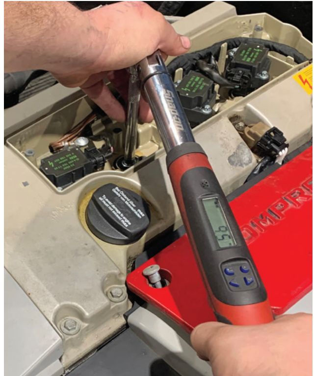
Proper torque is critical to spark plug seating! It only takes a few extra seconds and is the only way to do the job correctly.
