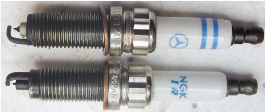
In this photo, an NGK spark plug is compared to a Mercedes-Benz spark plug. The Mercedes-Benz spark plug has the correct thread length for proper indexing and meets the correct heat range criteria.
