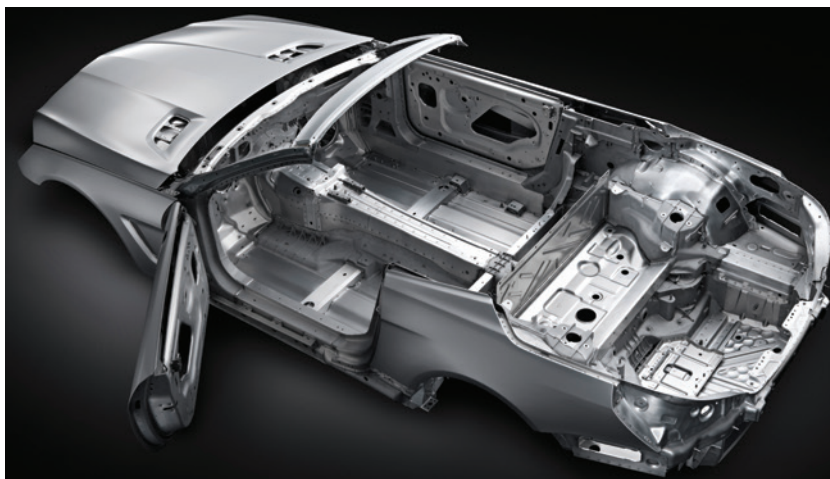
The aluminum-intensive R231 Chassis SL500 has extruded aluminum frame rails and longitudinal members, cast aluminum door sills, wheel wells, firewall, and strut towers, and aluminum sheet metal body panels. Some aluminum parts, including portions of the frame rail and the friction-stir-welded plate floor, can be installed only during vehicle production. The only non-aluminum structural component is the steel windshield frame.
