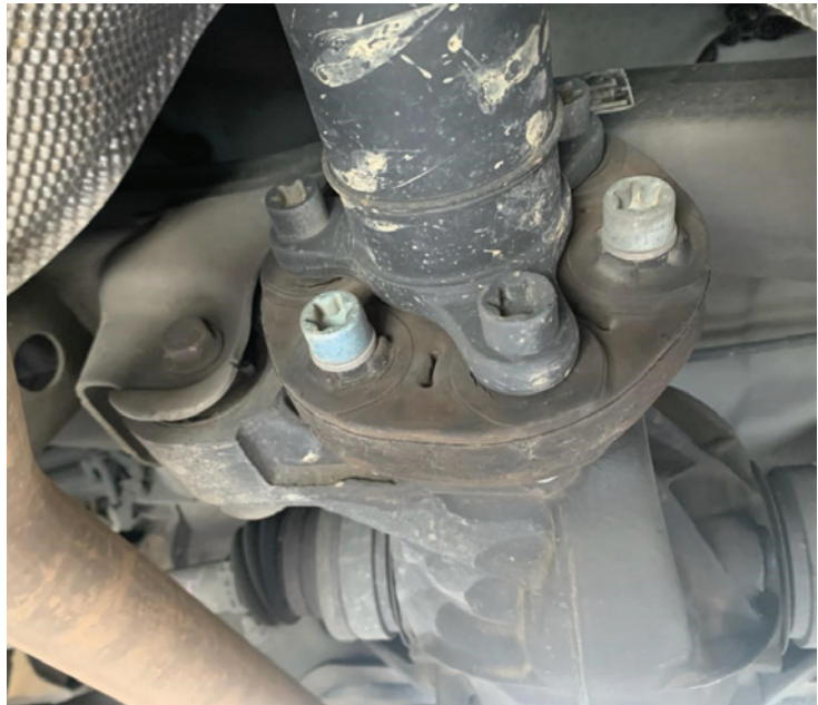
Be sure to check for cracks and loose bolts at the flex coupler, a sure cause for vibrations! Look closely and you'll see that this disk is cracked and needs replacement.
