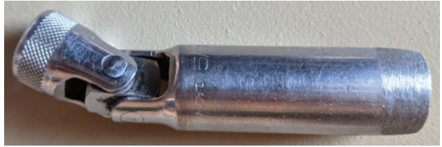
A quality spark plug socket with a swivel end helps in tight spots. Also be sure it has an internal grip to keep the plug from dropping into the spark plug well.
