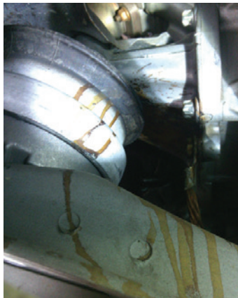
Note the leaking fluid from this engine mount. A damaged mount could be the cause of a judder complaint that the customer thinks is a transmission issue.
