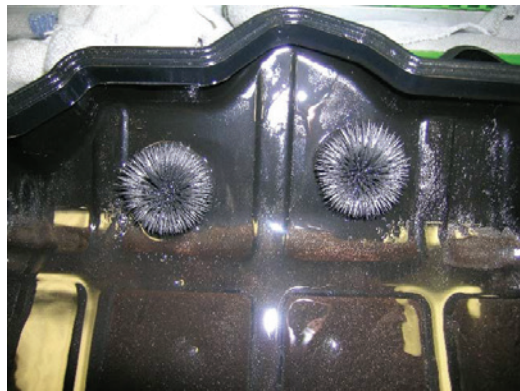
If you find a significant amount of metal in the pan and fluid, it may be time to replace the transmission assembly. This shows metal particles attracted to the magnets in the pan.
