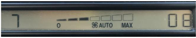
Here we see the diagnosis mode display code 7 showing a system high-side pressure of 8 bar. Since the engine is running and A/C is on, a low reading such as this indicates a low refrigerant charge, confirmed by noting the passenger-side vent is delivering cooler air than the driver-side vent.
