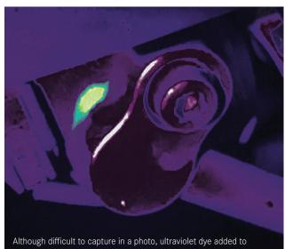
Although difficult to capture in a photo, ultraviolet dye added to the A/C system will help you find even the smallest leak with your eyes, here seen in green at the compressor connection.
