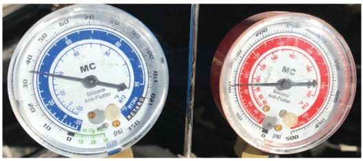
In the same car as the previous gauge photo, but with the engine running and A/C engaged, these gauges, with the high-side low and the low-side high, indicate a faulty A/C compressor.
