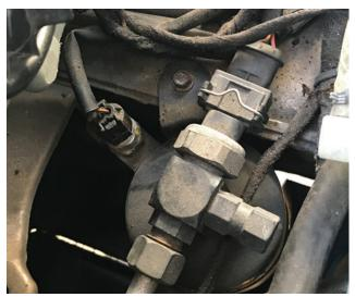
The refrigerant pressure (B12, top) and temperature (B12/1, left) sensors are both located on the receiver-drier, found behind the driver's headlamp. They are at system pressure, so be sure to evacuate and recover the refrigerant before loosening them.
