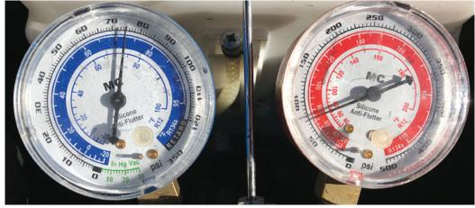
Old-school manifold gauges can be used to understand the problem. With the engine off, both gauges read the correct pressure corresponding to the system temperature (73°F, scale with white numbering for R134a), meaning the system is properly charged.
