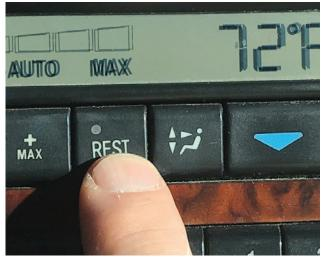
Pressing and holding the REST button on the climate control controller (N22) starts the diagnostic display mode. Diagnostics are best performed with the engine running.
