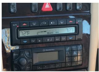
The climate control controller (N22) is located just above the radio in the center stack. Use the standard radio-removal tools to remove N22 from the dash.
