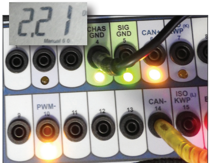
CAN low, ECM disconnected
