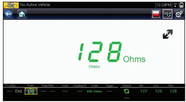
Figure 8: CAN bus resistance ECM unplugged
