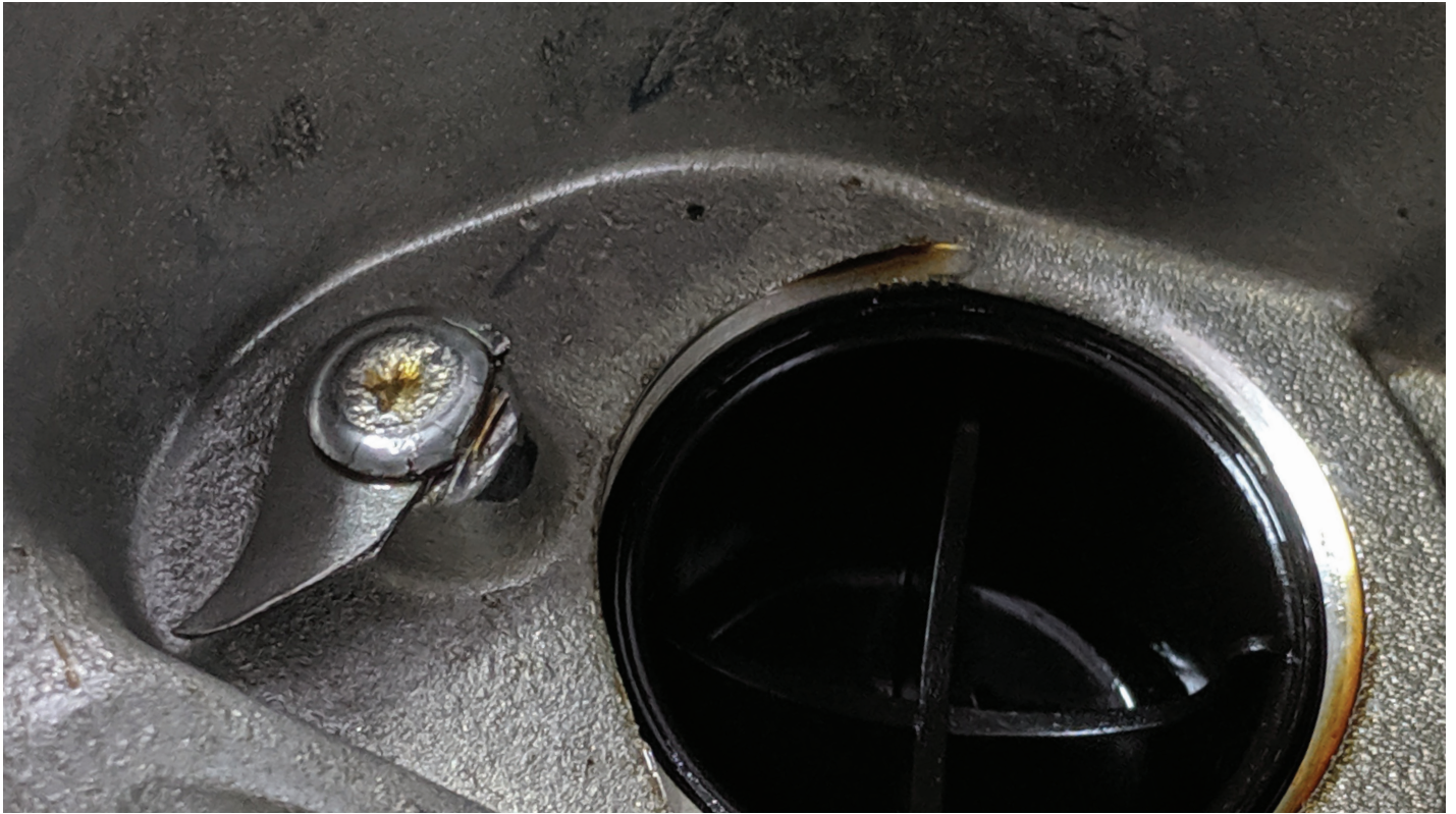
Only a small jagged piece of baffle was left on one of the rivets.
