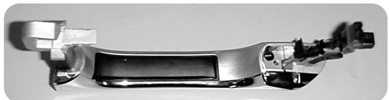
A door handle equipped with KEYLESS GO. Note the black micro switch on the inside of the door handle for unlocking and the dark sensor on the outside for locking and operation of the windows.
