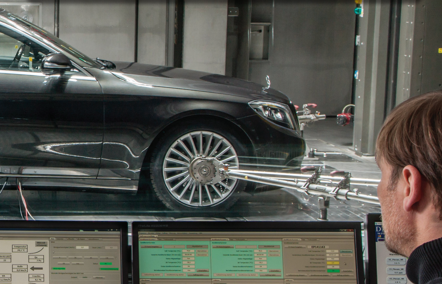
Shown here: Mercedes-Benz S-Class with the R744 CO 2 air conditioning system in a wind tunnel test.
