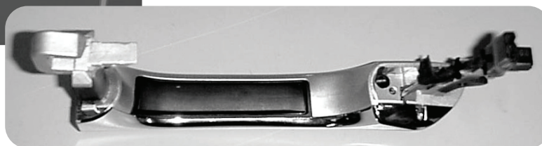
A door handle equipped with KEYLESS GO. Note the black micro switch on the inside of the door handle for unlocking and the dark sensor on the outside for locking and operation of the windows.
