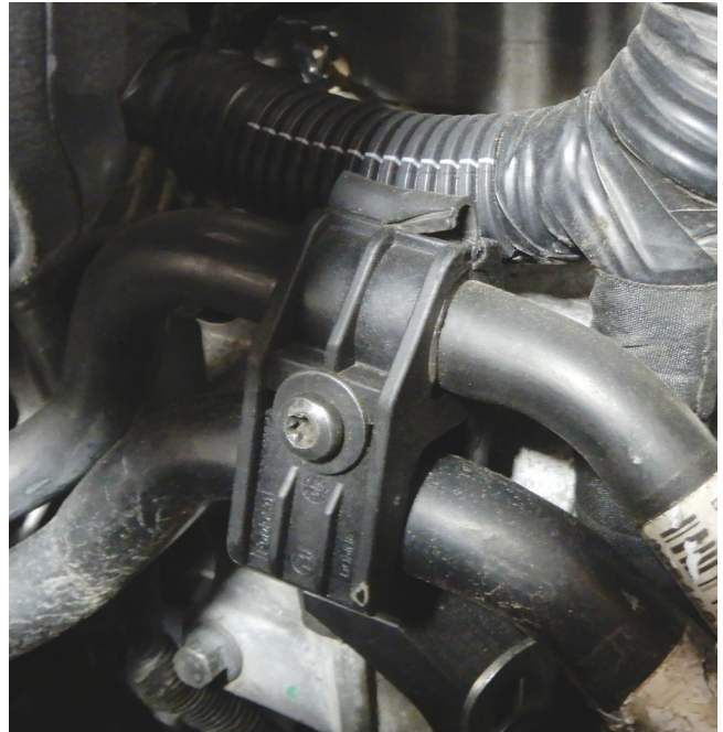
T30 Torx bracket for air conditioning lines
