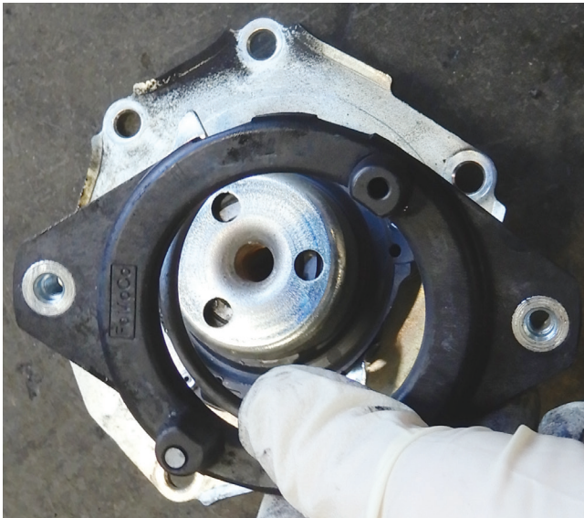
Water pump with spring assembly
