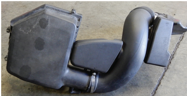
Air filter housing with fresh air tube
