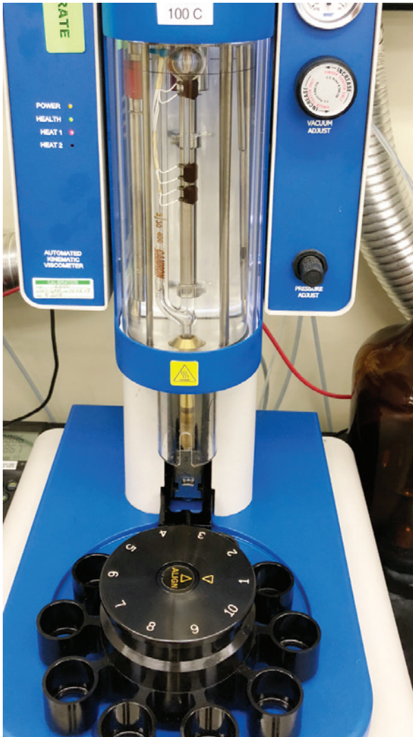
The device here is an advanced automatic kinematic viscometer as shown in Castrol's testing laboratory. This instrument is used to measure the high temperature viscosity of oil measured per ASTM standard D445.
