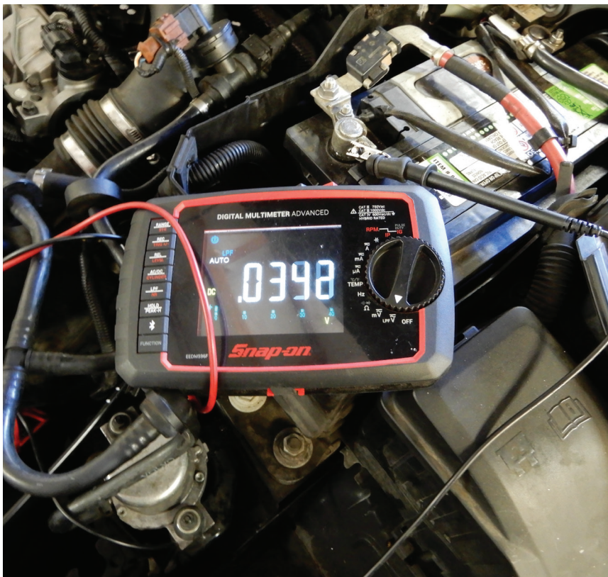
Checking voltage drop between the battery and the alternator using a multimeter
