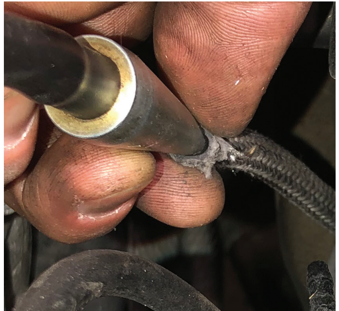
Applying pressurized smoke past the electric solenoid to the wastegate actuator
