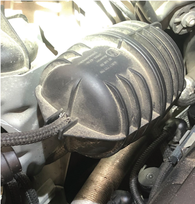
These plastic tanks hold vacuum for a constant supply when needed. Many line connections and bends equals possible failure/leaks.
