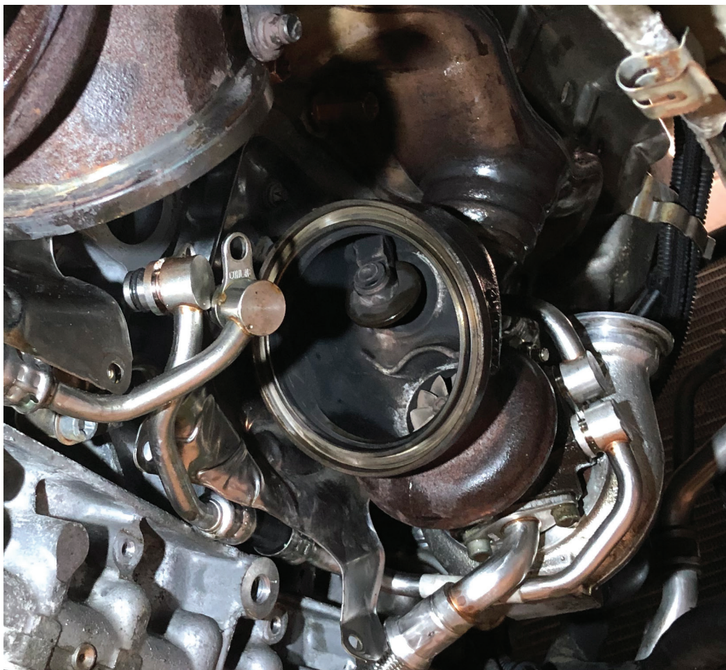
Both turbos installed with catalytic converters removed, provided access to the wastegate valve.
