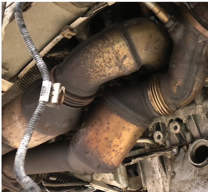
Catalytic converters mounted to turbochargers with subframe removed
