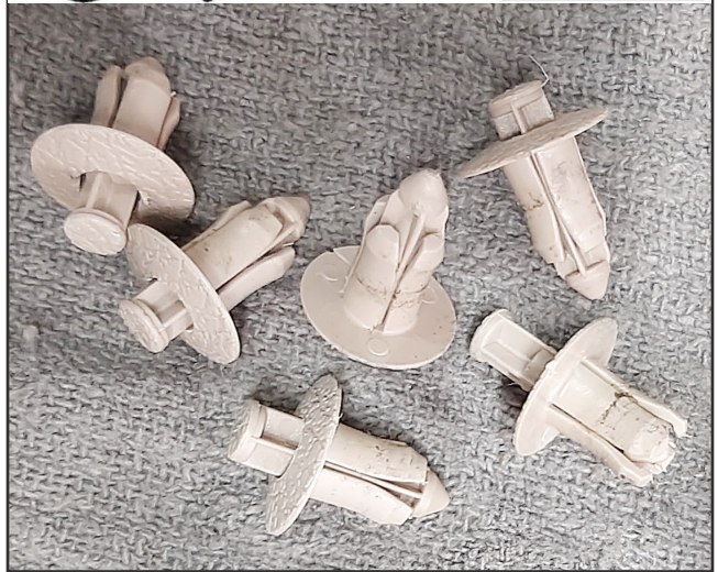
Remove the six press clips at the bottom edge of the door.
