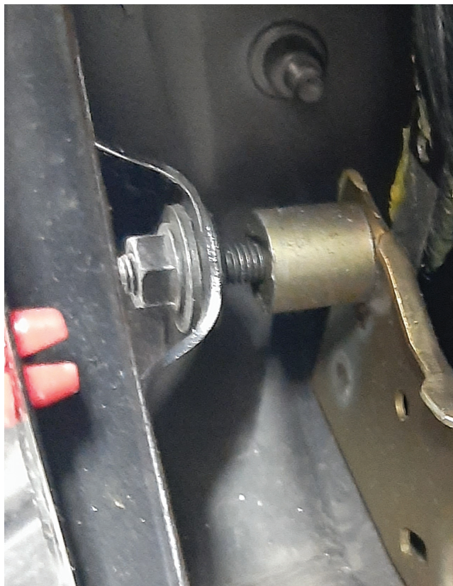
Front window cassette adjustment bolt
