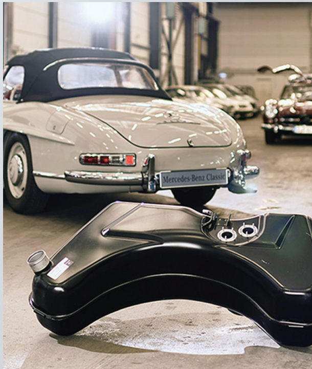
The Mercedes-Benz Classic Center specializes in both hard-to-find and common parts for older models. Here we see a fuel tank for the W198 Gullwing.
