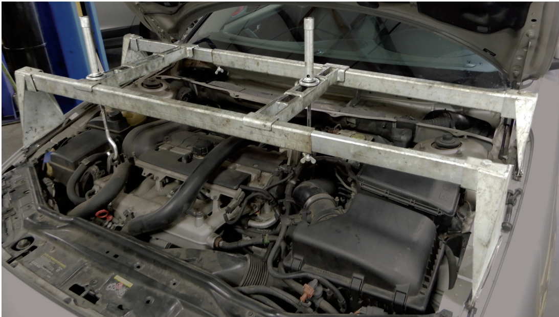
Special tools number 9995460 and 9995716 holding up the engine and transmission
