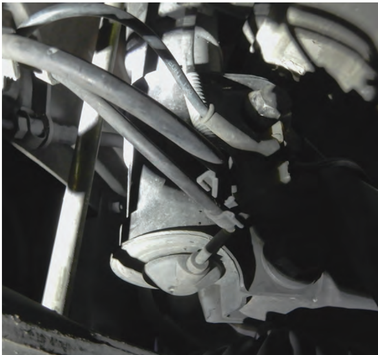
2006 Volvo S60R front and rear struts with electrical connections
