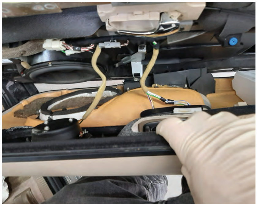
Lift up on the door panel.
