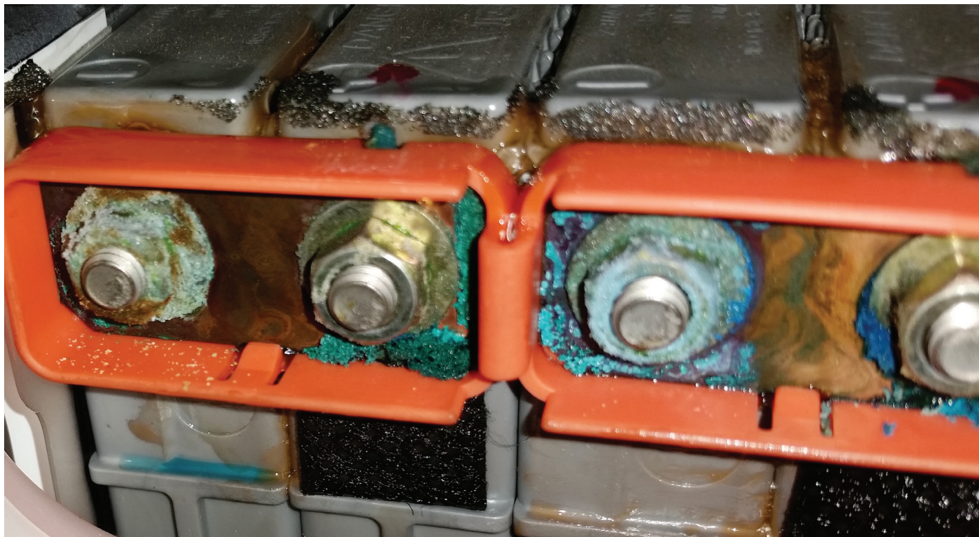
This 18-year-old Prius battery is leaking electrolyte from the battery terminals (note the plug liquid below the first terminal). The foam air dam on the battery cover was soaked in electrolyte and caused a loss of isolation.
