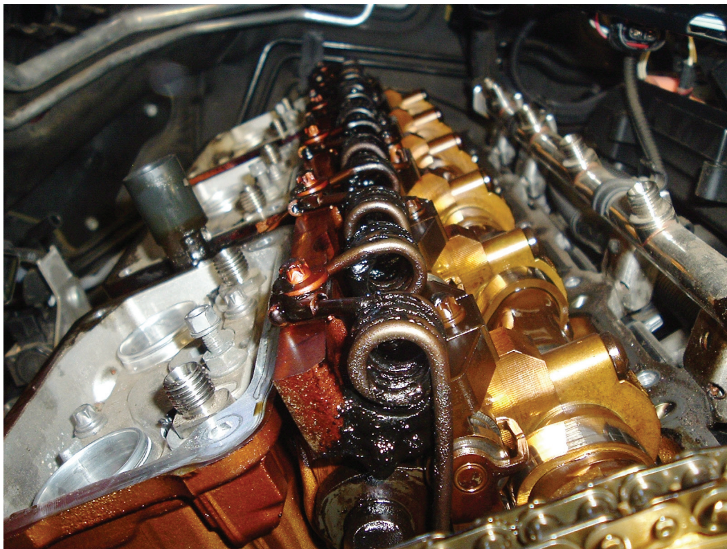
This valve cover was removed from an N55 engine with only 55k miles. Note the sludge buildup already. The customer had the oil changed at the dealer at the recommended intervals of 15k miles. Not often enough!
