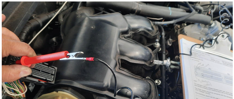
Figure 13: The headlamp doesn't illuminate when checking Pin 46.
