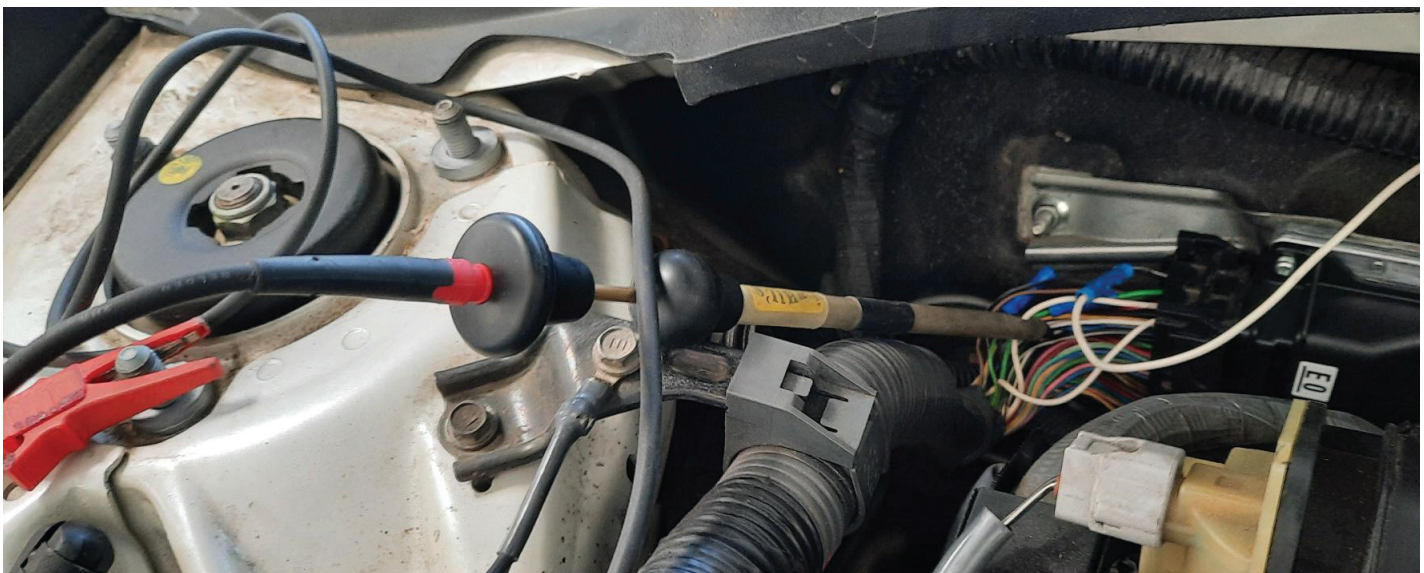
Figure 15: Applying temporary ground with my Phil's Probe. I don't like to flow current through the Phil's Probe as too much will burn off the needles, but I'm going to risk that the pulse width modulation of the sensor will not burn the needles (and it didn't.)
