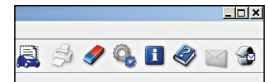
Figure 6: The menu at top right shows icons (from left to right) that open the Vehicle Data Card; print the current document; erase the current VIN and clear the screen; display the model designation; display the current search context; open the online help system; display system messages; and start the WIS Feedback system, allowing you to report errors you find.
