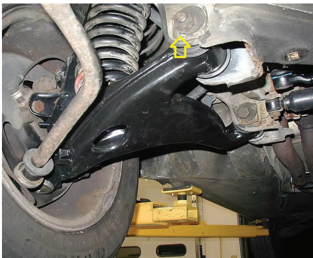
You won't see many of these style control arms anymore! Note the adjustment cams.
