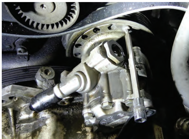
Be sure to install the drive belt when reinstalling the power steering pump. Otherwise, you'll have to pull it back apart.
