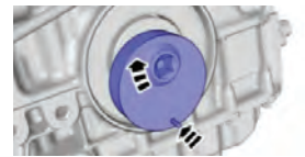
Volvo special tool 9997257 mounts on the front of the engine.
