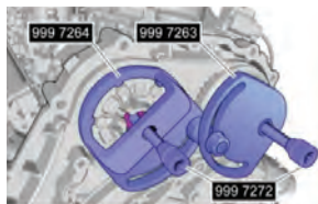
Three special tools are needed for removing the timing gear sprockets.
