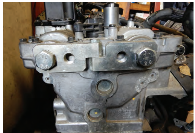
You need to lock the two camshafts into position using special tool 9997261.
