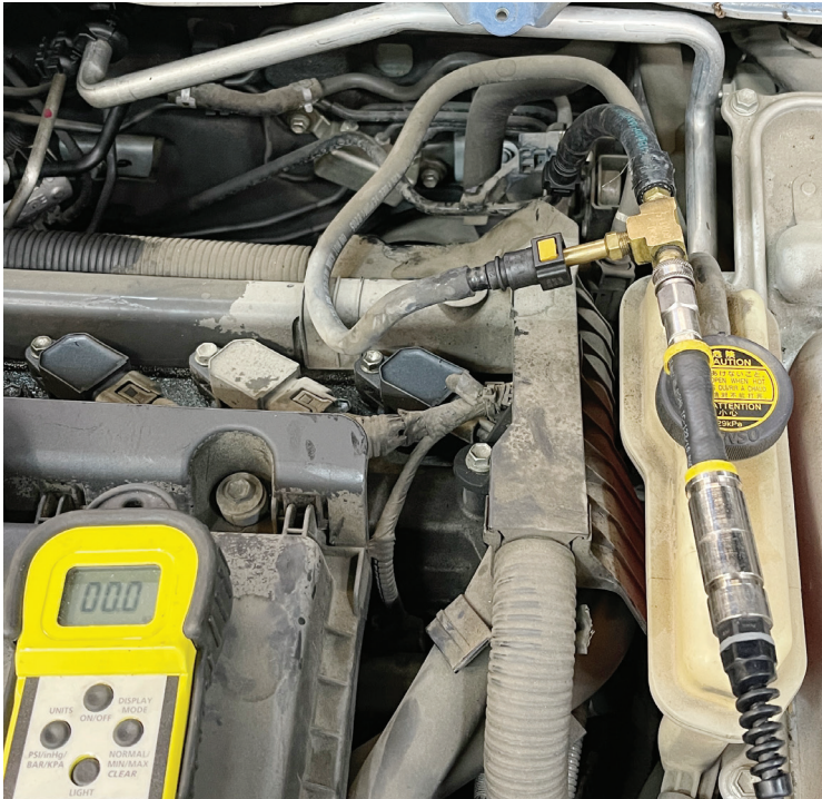
Fuel pressure at zero
