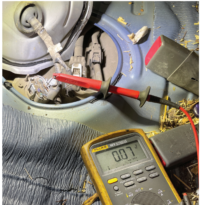
Ground OK at fuel pump
