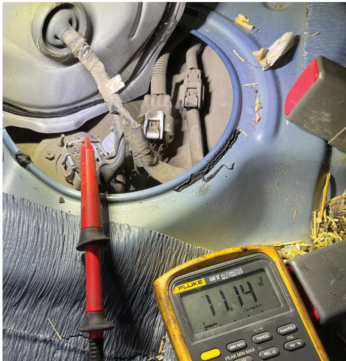
Power OK at fuel pump
