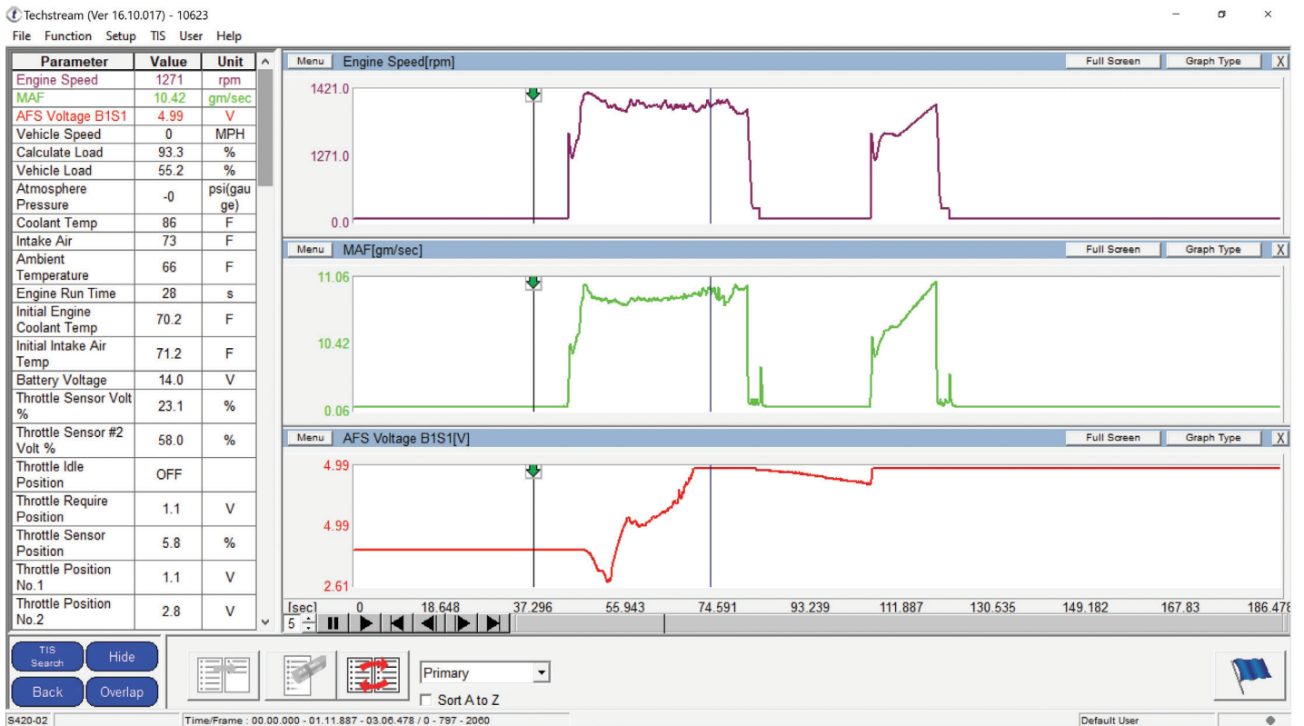
Live data during cranking
