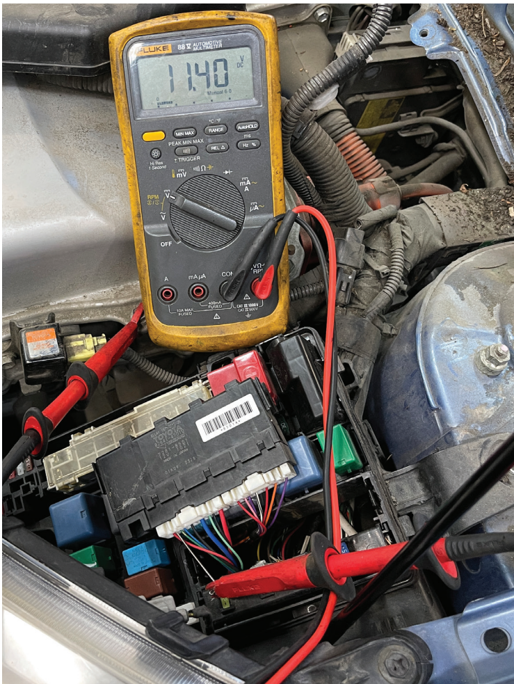
Testing power at the fuel pump relay
