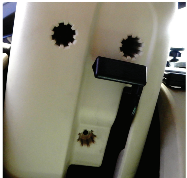
At the bottom trim at the steering column, remove three screws.
