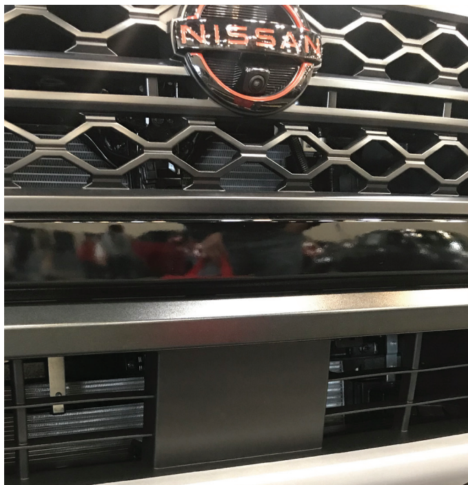
Front Radar - Intelligent Cruise Control Sensor
