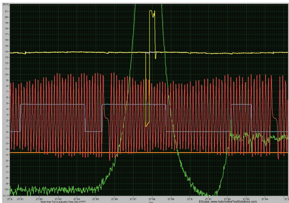
Figure 1: A signal overlay of crankshaft sensor, camshaft sensor and in-cylinder pressure waveform with ignition signal. This MASINT setup is what we use to check ME-SFI signal timing against mechanical engine movements.
