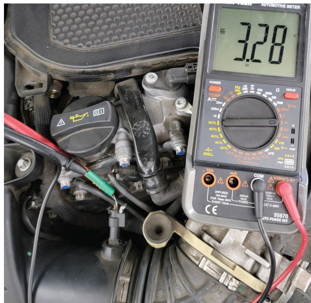
Figure 3: The IAT signal voltage running normally on our E350 on this 76-degree day at a client's shop in California. This voltage checks good based on the service information.
