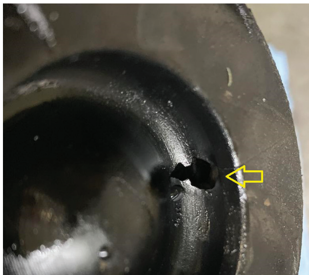
There are times when something external causes the damage. This piston damage may have been caused by an overaggressive tune chip. Mercedes-Benz does not support the use of aftermarket tuners.
